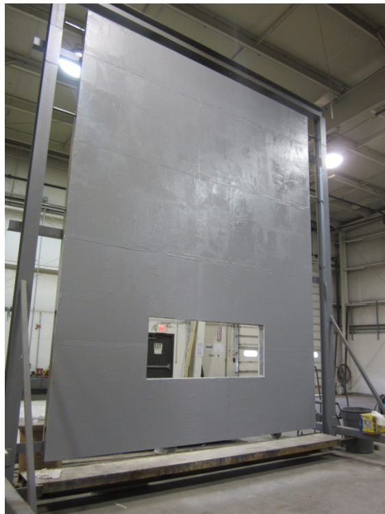
Photo No. 6 Complete Air/Vapor Barrier www.archtest.com
