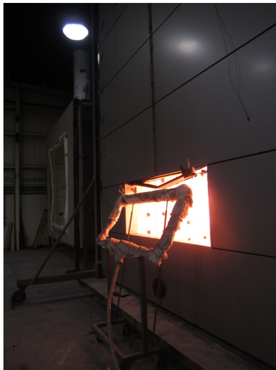
Photo No. 14 Window Opening Header Trim Buckling
