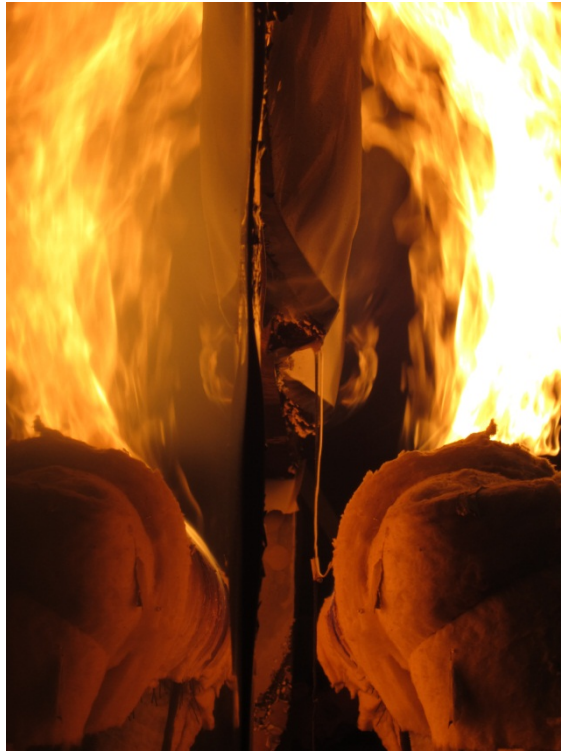
Photo No. 17 Ignition at Window Opening Header
