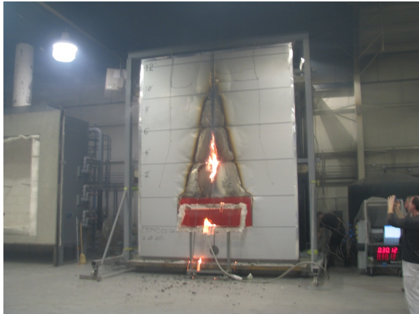
Photo No. 18 Room and Window Burners Extinguished
