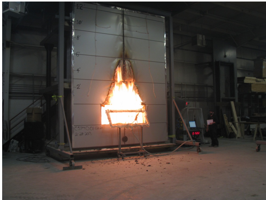
Photo No. 16 Assembly Halfway into Flame Duration
