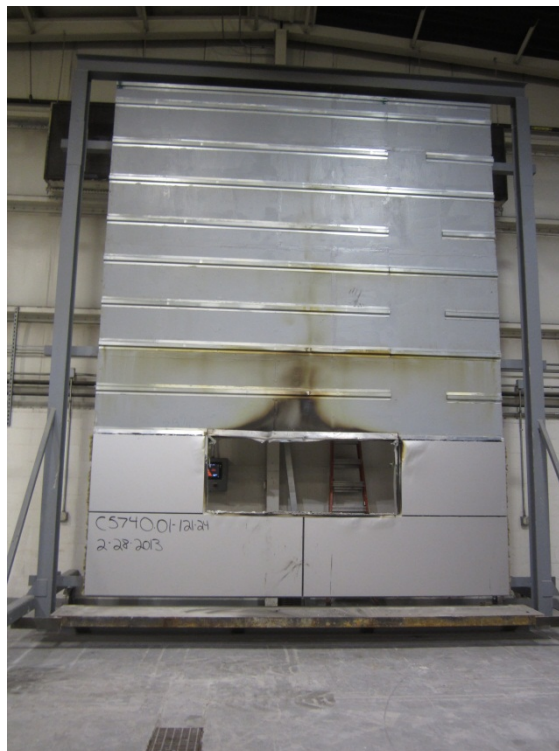
Photo No. 20 Panels Removed (Post-Test)
