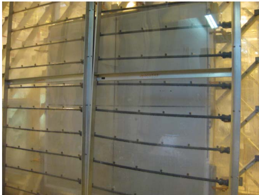
Photo No. 2 Water Penetration Test
