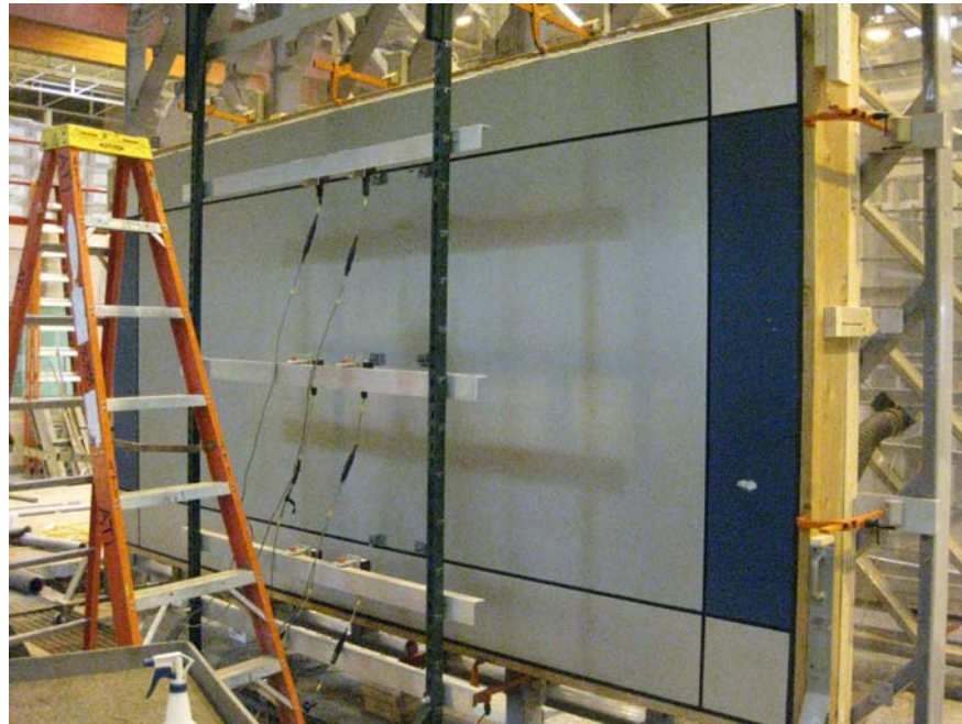
Photo No. 3 Full System Structural Load Test Set-up
