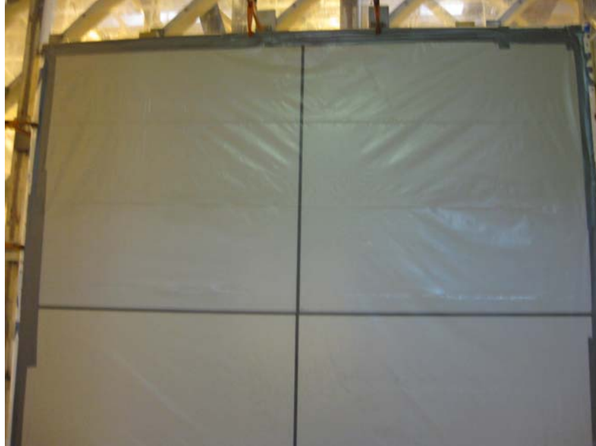
Photo No. 1 Air Infiltration Test with Tare Bag
