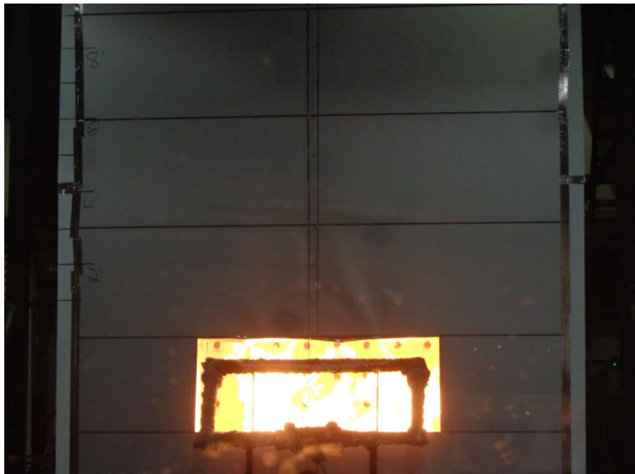
Photo No. 12 Panels Warping
