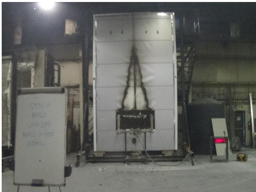
Photo No. 16 Complete Assembly (Post-test)
